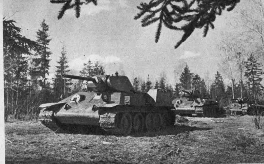
Russia's great medium tank, T-34, is the world's outstanding example of the use of Christie-type suspension, an American design more than 25 years old. This suspension is characterized by large, evenly spaced bogie wheels touching top and bottom of track.
